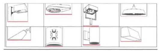
(b) Fixtures not fully shielded. Even though the lamp is shielded from direct view from the side or above, reflective surfaces within the fixture and/or lens covers are directly visible from the side.
